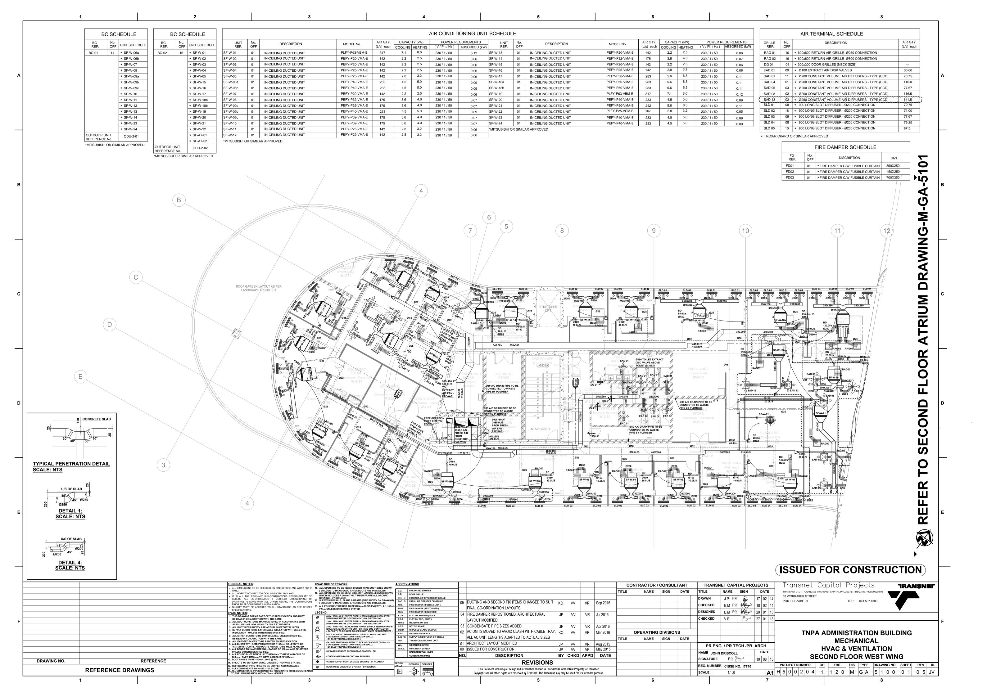
AIR TERMINAL SCHEDULE GRILLE No. REF. OFF AIR QTY. DESCRIPTION (L/s) each RAG 02 04 \*600x600 RETURN AIR GRILLE -Ø300 CONNECTION SAD 14 01 \*Ø250 CONSTANT VOLUME AIR DIFFUSERS - TYPE (CCD) SAD 07 07 \* Ø250 CONSTANT VOLUME SWIRL AIR DIFFUSERS-TYPE (CSW) 87.5 \* TROX/RICKARD OR SIMILAR APPROVED
